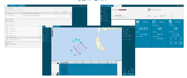
SEAPLAN software developed by SEABER, is an ideal and versatile interface to set up mission and monitor YUCO micro-AUV. It allows to create waypoints and segments fully settable (speed, depth, latitude, longitude, etc) in order to create missions. The AUV Dashboard allows to monitor YUCO micro AUV and to display faults and their resolutions. Logs are exported under .CSV format.
